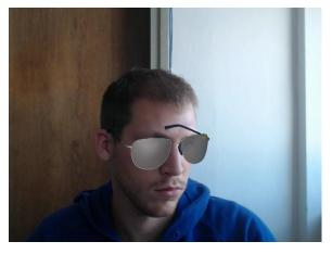
In reality, parts of the glasses are occluded by the head, nose or ears. To achieve the same effect in augmented reality, an occlusion mask is used. This is an object shaped roughly like a human head and placed inside the glasses. At runtime, the occlusion mask covers the object behind it but is not itself visible, achieving the desired effect. This is achieved using material settings for the occluder object.
